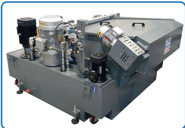
Filtering system below the bar loader
